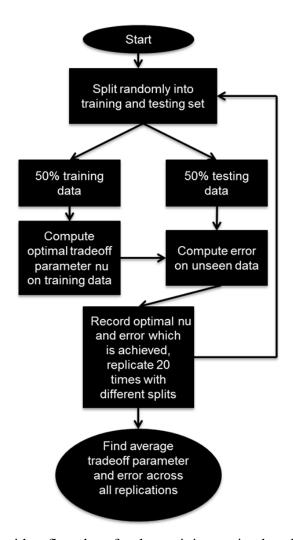
Figure 10: Algorithm flowchart for determining optimal trade-off parameter
