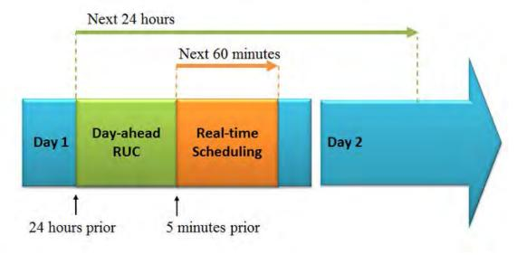
Figure 26: Two-layer dispatch model
