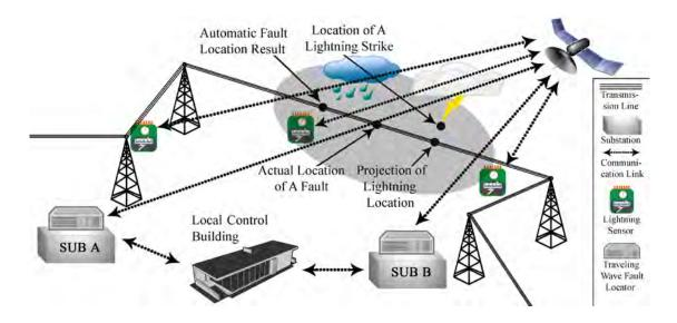
Figure 5: Spatio-temporal correlation of traveling wave fault locator data with lightning, GIS and GPS data
