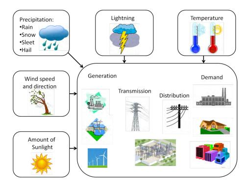
Figure 1: Weather factors affecting power system
