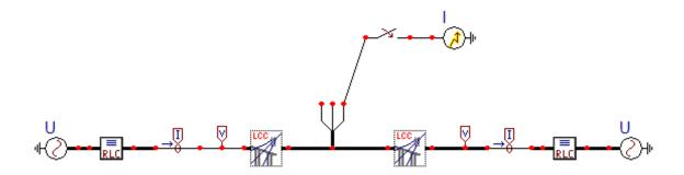
Figure 2: ATPDraw model of the tested line
