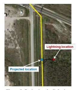
Figure 9: Projecting the lightning
