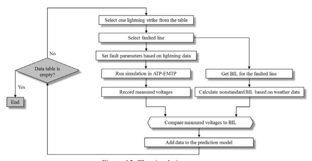
Figure 15: The simulation process
