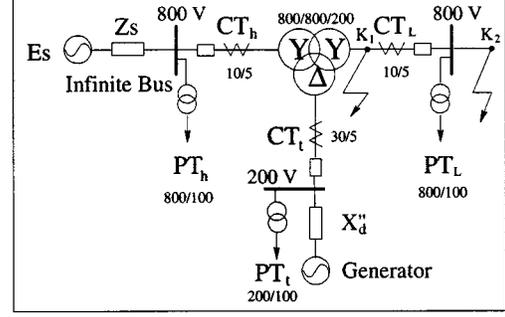
Fig. 1. Reduced equivalent diagram of the EPDL system.
