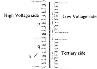
Fig. 2. Turn-to-ground fault.
