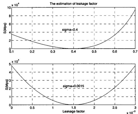
Fig. 4. Summation voltage versus leakage factor.
