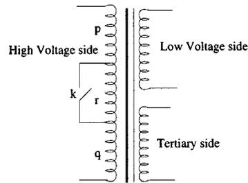
Fig. 3. Turn-to-turn fault.
