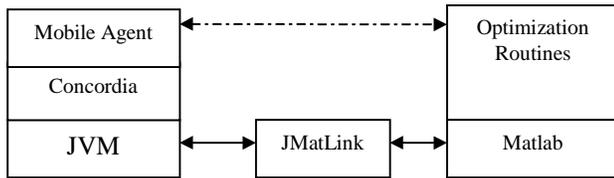
Figure 6. Links between JVM and Matlab
