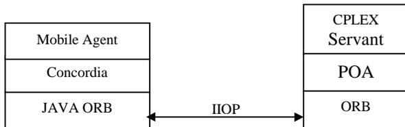
Figure 7. Calling CPLEX using IIOP
