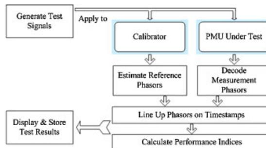
Figure 8. Framework of step test programs.
