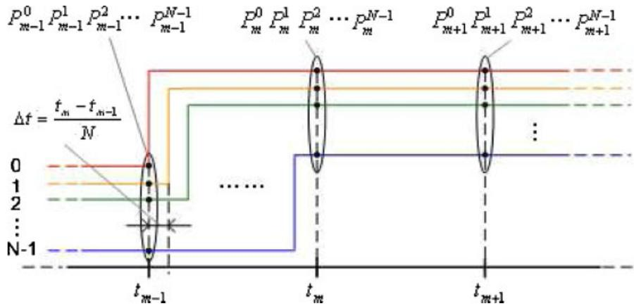
Figure 3.  $N$  sets of output phasors obtained by repeated measurements of time-shifted step signals.
