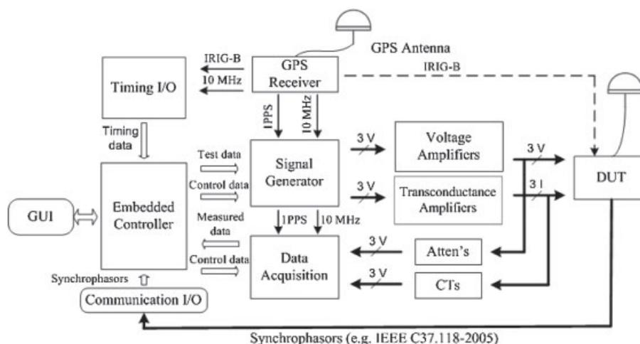
Figure 7. Diagram of the step test system.
