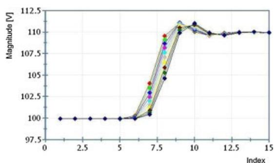
Figure 5. Output phasors of a PMU before interleaving.
