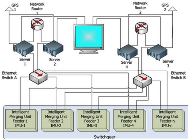
Fig. 2. Server based CPC system [11].
