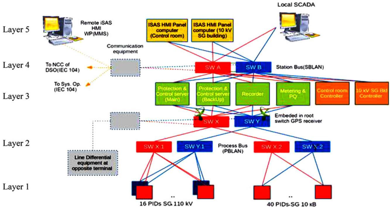
Fig. 4. The PACS structure of 110/10 kV “Olympic” substation in Northwest Siberia, Russia [15].
