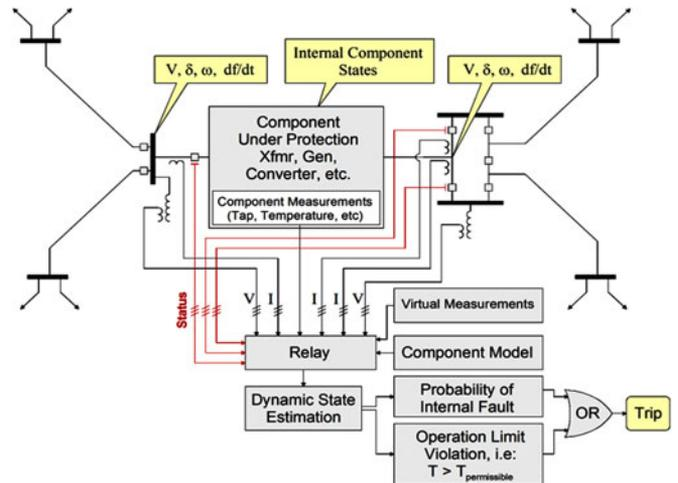
Fig. 5. DSE-based protection embedded in CPC.
