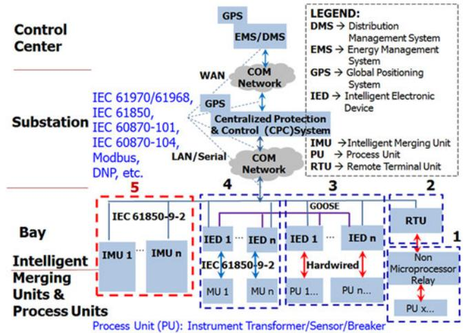
Fig. 1. Evolution of protection, control, monitoring and communication system leading to CPC [11].
