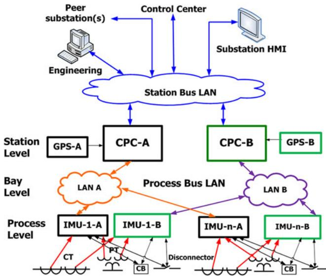
Fig. 3. One CPC architecture in a substation (Architecture 5a, [1]).
