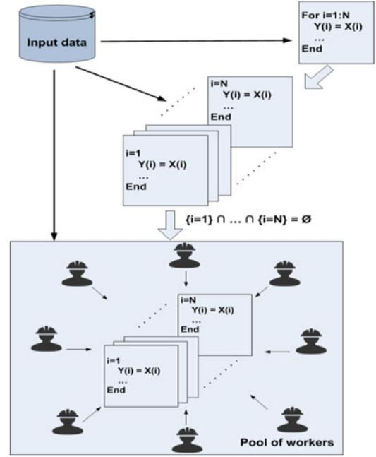
Fig. 3. General implementation of parallel computation for N tasks.
