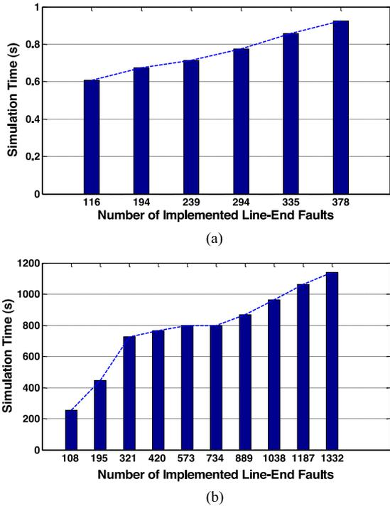
Fig. 7. Simulation time based on the required number of line-end faults; (a) Case ranked 1st in Table I in IEEE 118-bus system; (b) Case ranked 1st in Table I in Alberta transmission operator system.
