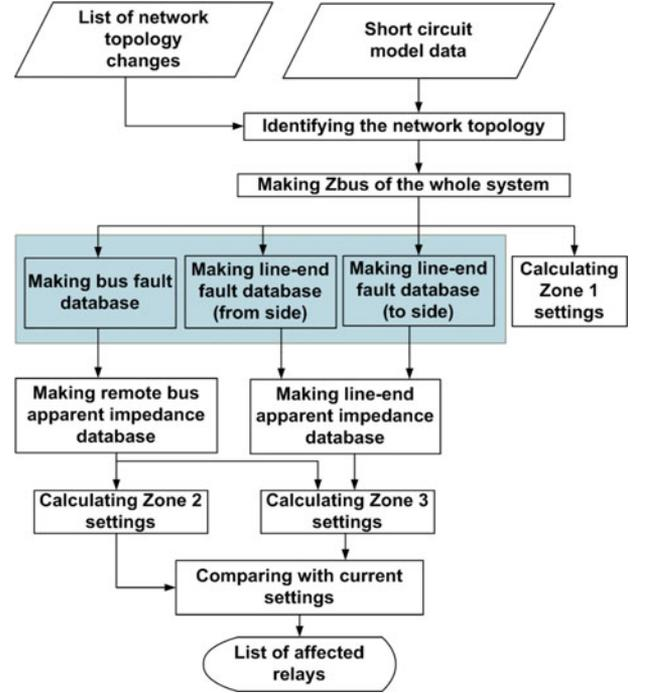
Fig. 2. General flowchart of the relay setting calculation module.
