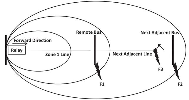
Fig. 1. Fault types used for phase distance setting calculation: remote bus fault (F1), next adjacent bus fault (F2), and line-end fault (F3).
