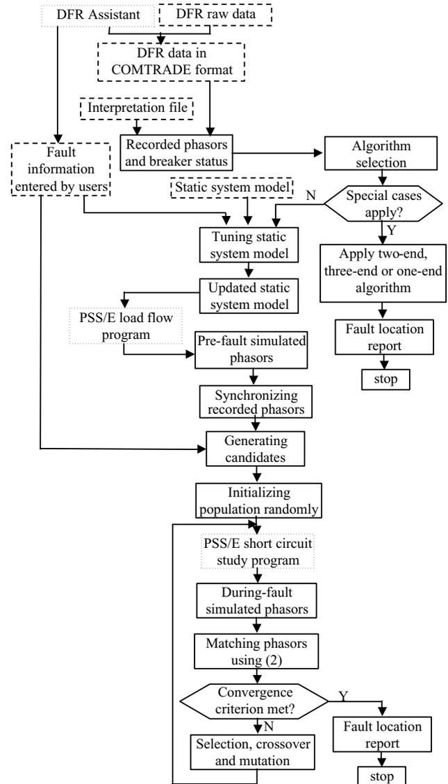
Fig. 5. The flowchart of fault location software.
