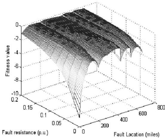
Fig. 2. The fitness surface for an A-G fault.
