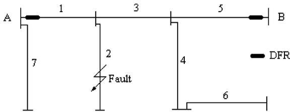
Fig. 6. Illustration of the building of the initial faulted branch candidates.
