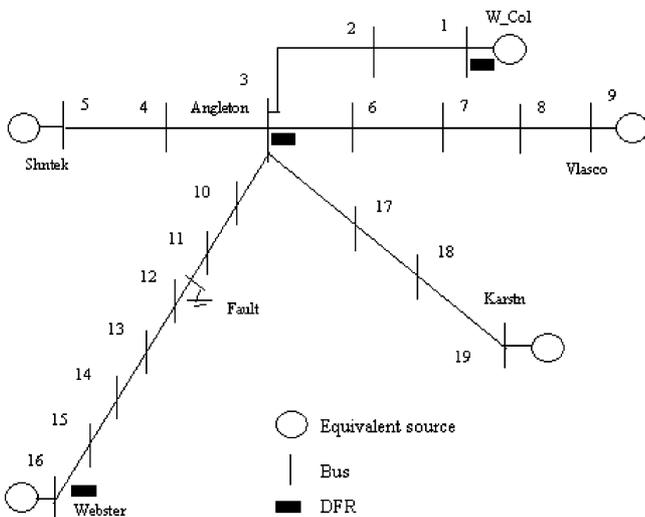
Fig. 1. The sample system for illustrating data sparsity.
