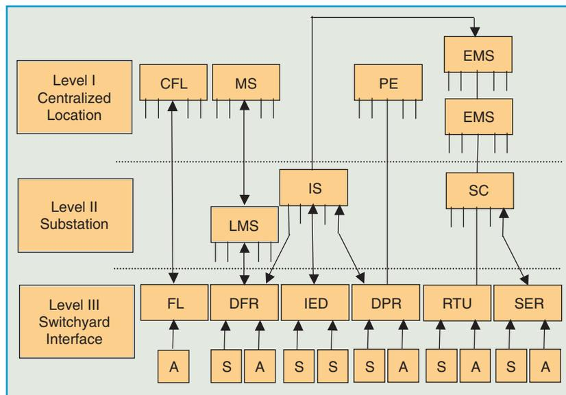
**figure 1.** Layout of the typical substation equipment (monitoring, control, and protection). FL: fault locator, DPR: digital protective relay, DFR: digital fault recorder, RTU: remote terminal unit, IED: intelligent electronic device, SER: sequence of events recorder, EMS: energy management system, PE: protection engineer, SC: substation control, IS: integrated system, CFL: central fault location, LMS: local master station, A: analog, S: status.
