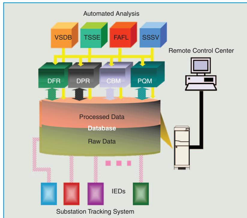
**figure 2.** One example of new substation functions supporting new applications. VSDB: verification of substation database, FAFL: fault analysis and fault location, TSSE: two-stage state estimation, SSSV : substation switching sequence verification.
