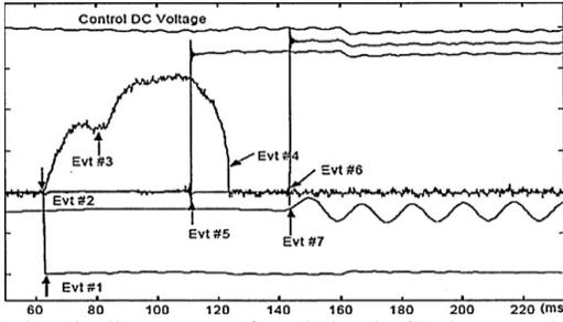
Fig. 2. Monitored coil current waveform during the CB close operation [27].
