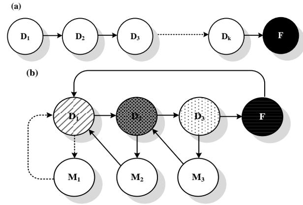
Fig. 1. (a) Classic state diagram for a deteriorating component over time; (b) 3-state deterioration/recovery state diagram with maintenance effects [30].
