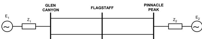
Fig. 3. Model of WAPA Glen Canyon-Flagstaff Power Network Section
