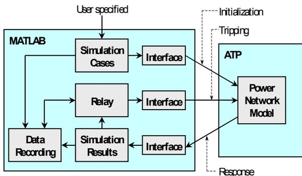
Figure 4. An Example of Integrated Simulation Tools for Protective Relaying by Using MATLAB and ATP
