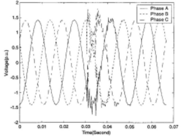
Fig. 8: Switching transient disturbance
