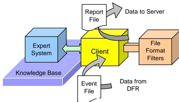
Figure 3: The architecture of Client
