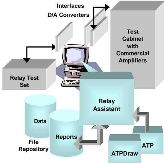
Fig. 4: The architecture of the simulator
