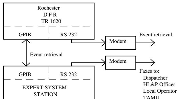
Figure 5. Final Expert System Configuration
