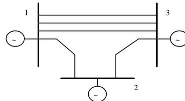
**Figure 9. One line diagram of the 161 kV power system used for EMTP modeling**
