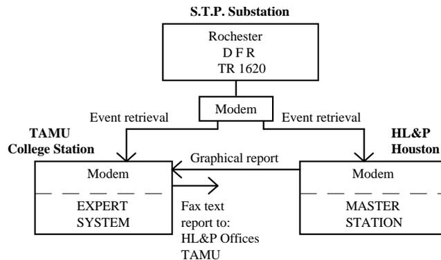
**Figure 4. Initial Testing Configuration**
