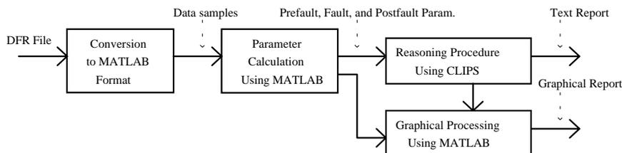
Figure 1. Expert System Block Diagram
