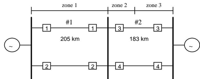
**Figure 10. One line diagram of the 345 kV power system used for EMTP modeling**
