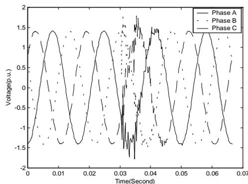
Fig. 3. The recorded switching transient waveforms
