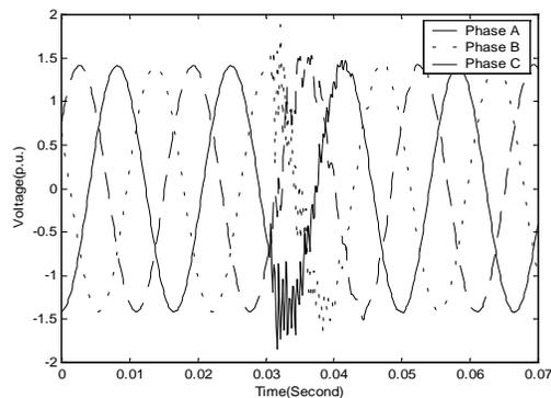
Fig. 4. The simulated switching transient waveforms
