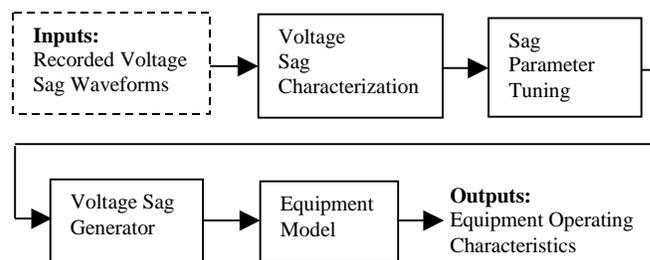
Fig. 5. The overall structure for equipment behavior evaluation
