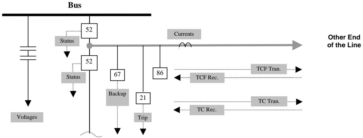
Fig. 1. Typical Breaker-and-a-half Bus Arrangement
