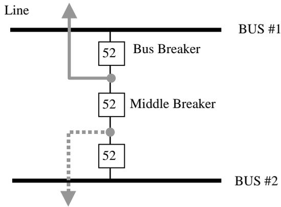
Fig. 2. Typical STP Bus-Breaker Arrangement
