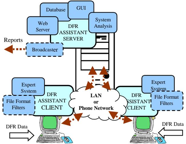
Fig 6. Architecture of the Installed System
