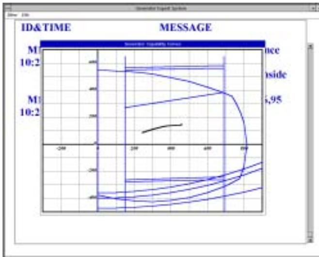
**Fig. 10. Generator capability monitoring window**
