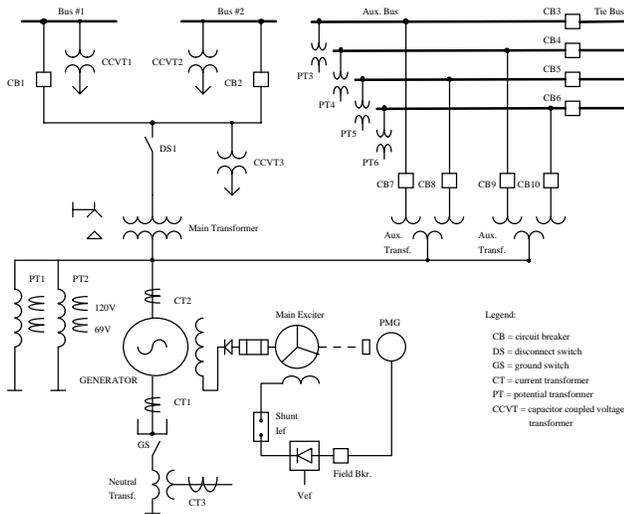
**Fig. 6. One line diagram of the power plant**
