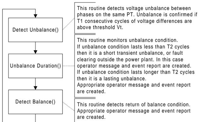
**Fig. 8. Logic for voltage unbalance (same PT) function**
