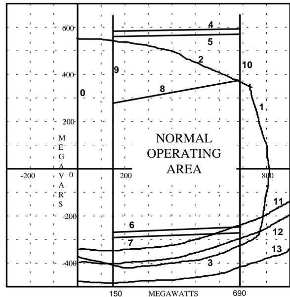
**Fig. 9. Generator gross capability settings**
