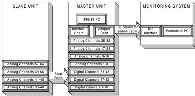
**Fig. 4. Communication interfaces for the DFR and external PC**
