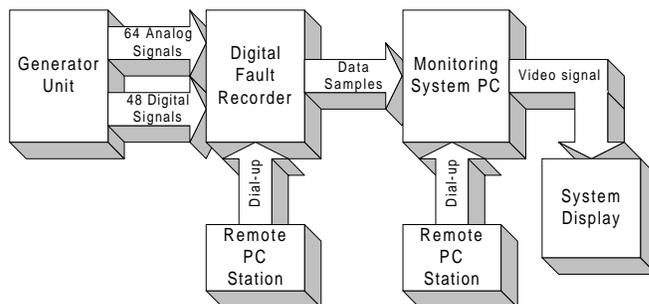
**Fig. 3. System's block diagram**
