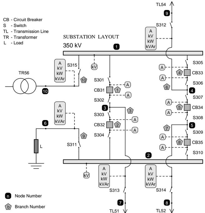
Fig. 1. One-line diagram of a typical substation layout with measurement device allocation
