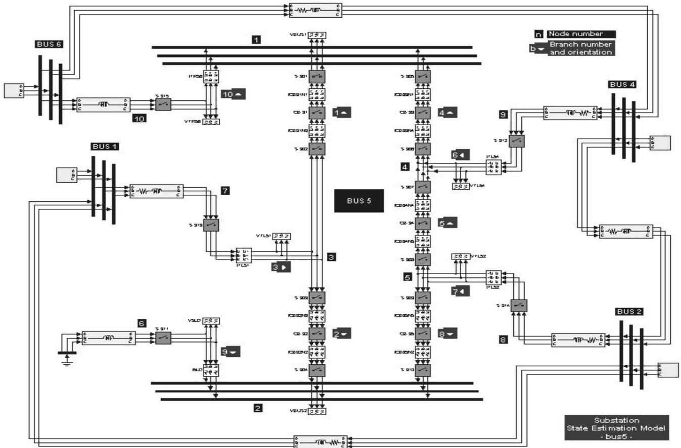
Fig. 2. Layout of the substation model as it appears in SIMULINK (comprising impedances that present boundary condition connections)
