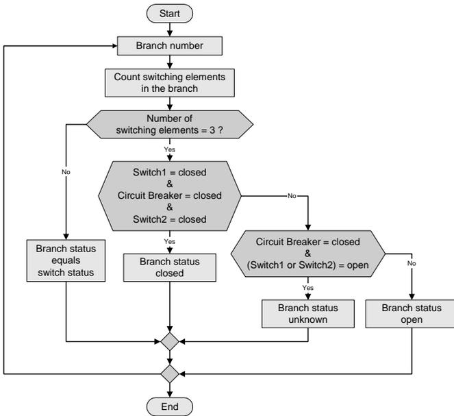
Fig. 5. Algorithm for branch status determination
