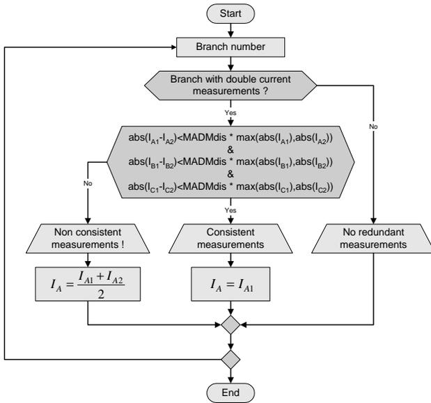
Fig. 3. Algorithm for checking the branch current consistency
