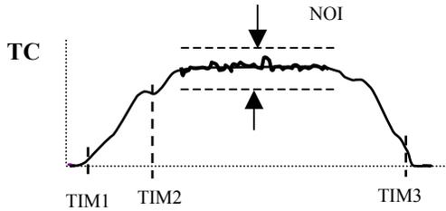
Fig. 2. Trip Current waveform and parameters
