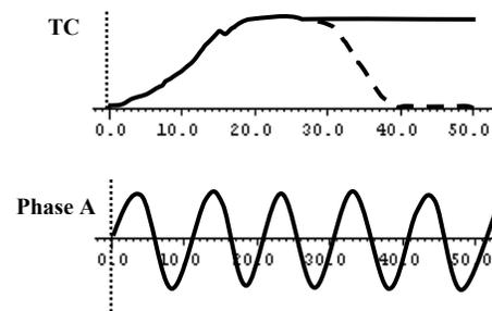
Fig. 6. Signal abnormalities for a stuck breaker
