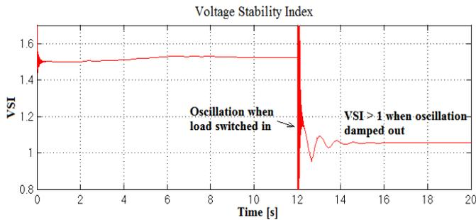
Fig. 7. Simulation results of SCIG-based wind farm with load and STATCOM
