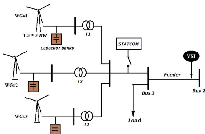
Fig. 3. Details of the SCIG-based wind farm and reactive power compensators
