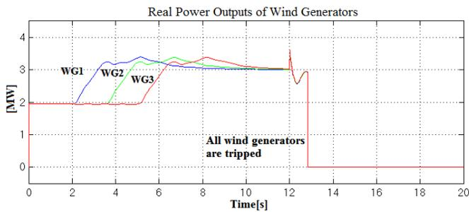
Fig. 6. Simulation results of SCIG-based wind farm with the AC undervoltage protection enabled
