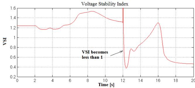
Fig. 5. Simulation results of SCIG-based wind farm with the AC undervoltage protection disabled
