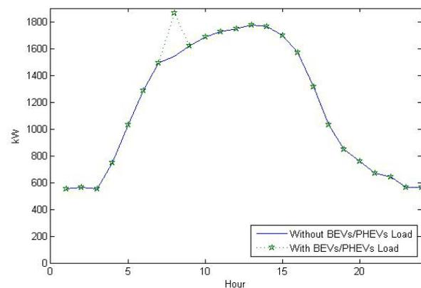
Fig. 3. Impacts of faster charging BEV/PHEVs on load demand.
