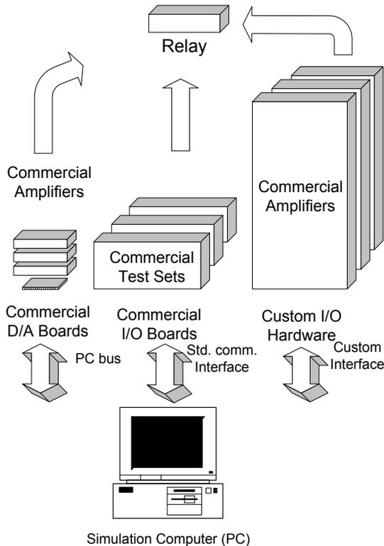
Fig. I. An advanced hardware configuration of an open-loop simulator
