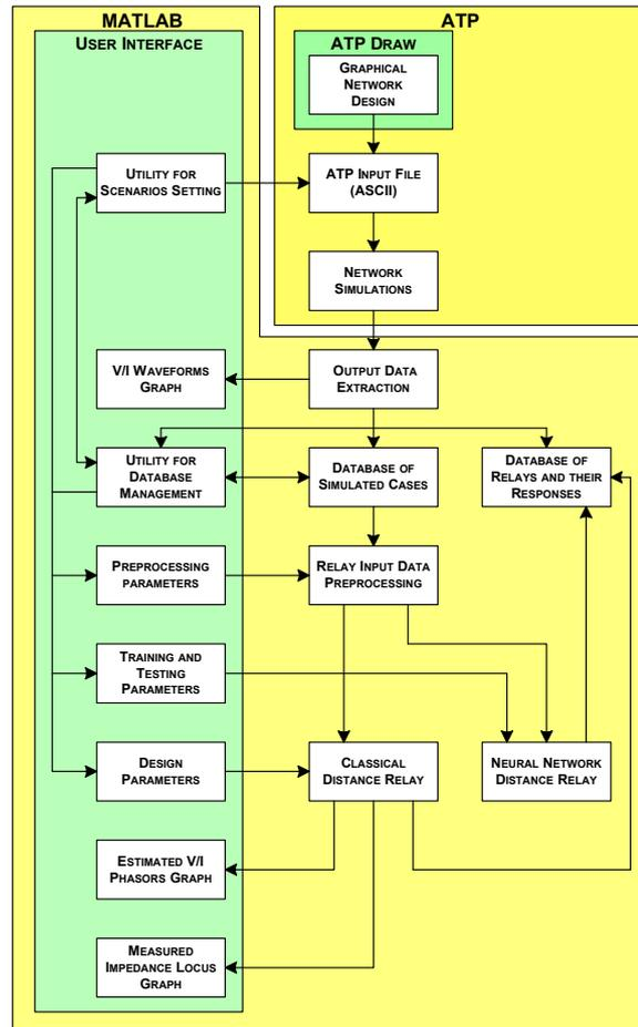
Fig. V. A new software for power system modelling and simulation as well as protective relay design and evaluation
