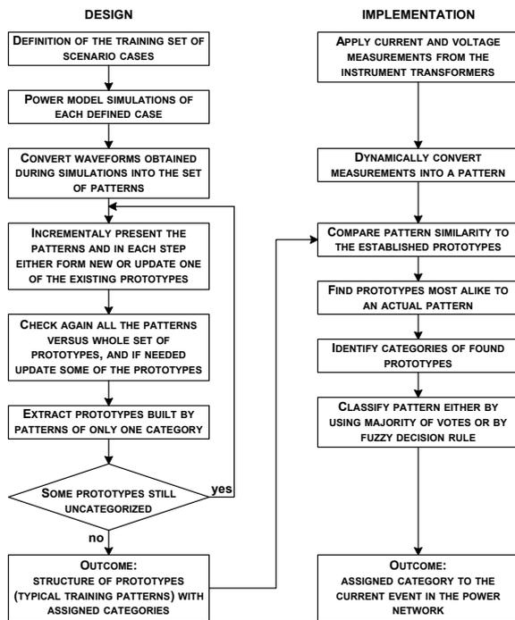
Fig. IV. Design and implementation steps of neural network based relay
