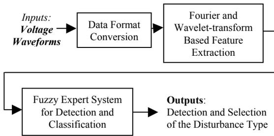
Fig. 4. Detection and classification flowchart
