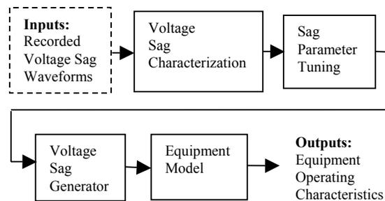
Fig. 5. The structure for equipment behavior evaluation
