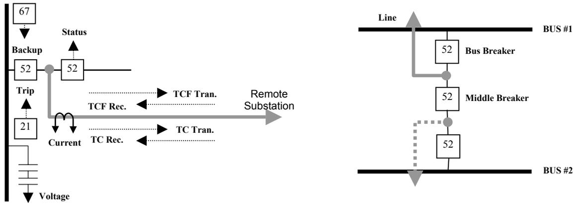
Fig. 1. An example of one line-diagram and the bus-breaker arrangement
