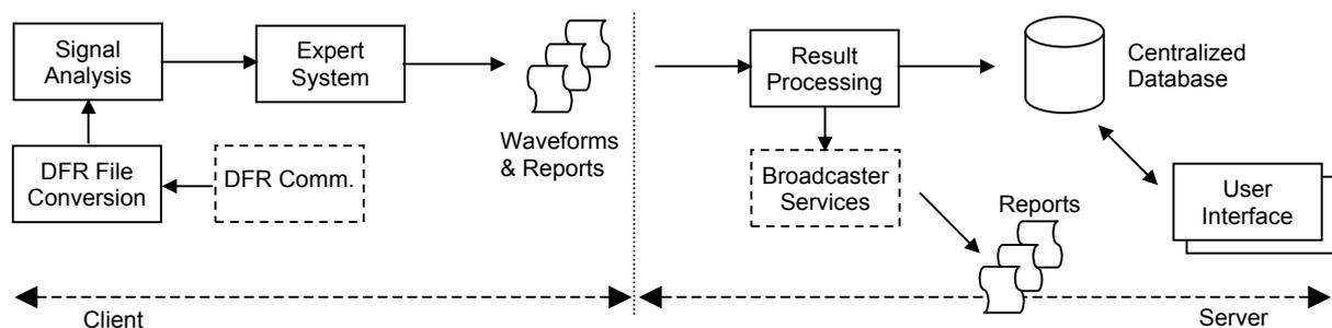
Fig. 2. Client/server architecture of the software for automated analysis
