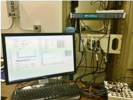
Figure 4. Reference PMU Test System at Texas A&M University
