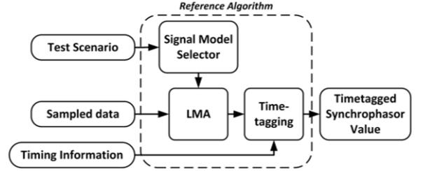
Figure 3. Procedure of synchrophasor estimation with proposed algorithm
