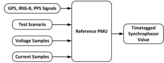
Figure 2. Input and Output of a typical Reference PMU
