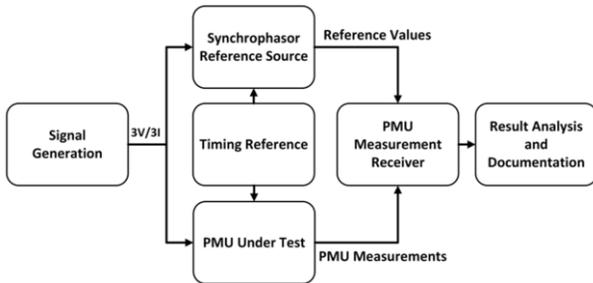
Figure 1. Structure of a typical PMU Calibration System
