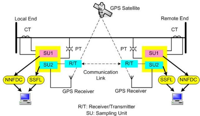
Fig. 3. Field configuration of combined fault analysis tool
