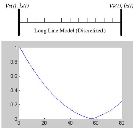
(a) Fault can be located when fault occurred within the primary line
