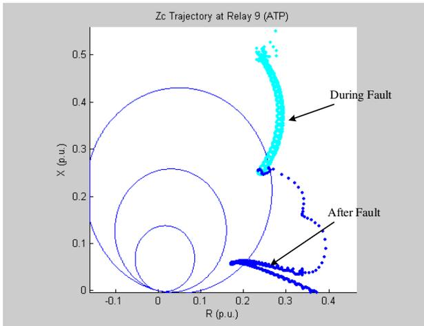
Fig. 9. Trajectory of computed impedance for distance relay of line 9-6 at bus 9
