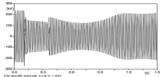
(a) Phase A voltage at bus 9 during the power swing
