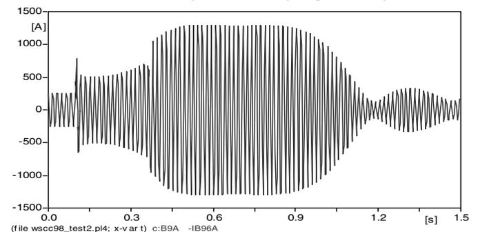
(b) Phase A current in line 9-6 during the power swing
