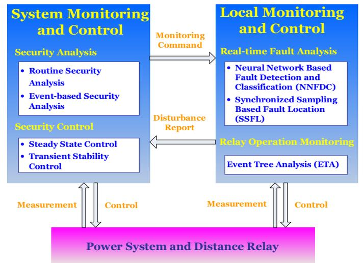
Fig 1. Interactive scheme for system-wide and local evaluation of impacts of relay operation
