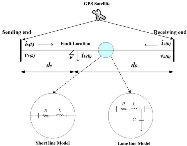
Fig. 4. An example of fault location calculated by SSFL
