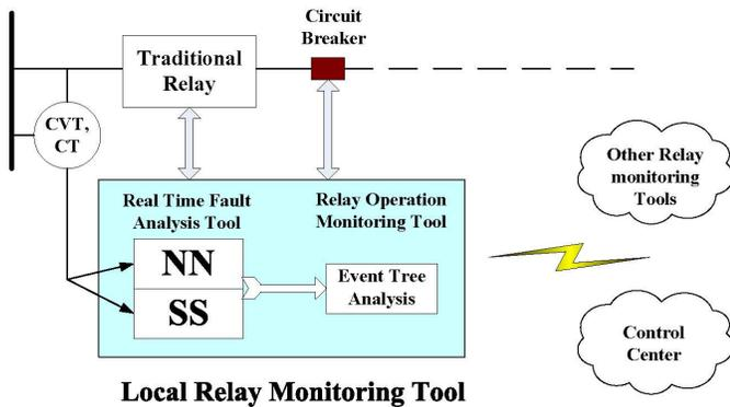
Fig. 2. Real time relay monitoring tool
