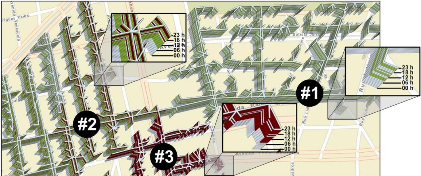
Fig. 6. Partial screen of the developed GIS application with tridimensional representation of risk levels hour-by-hour.
