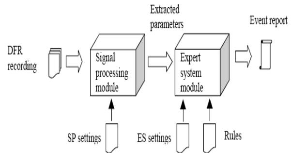
Fig. 3. Circuit Breaker Recorder Analysis Software Modules
