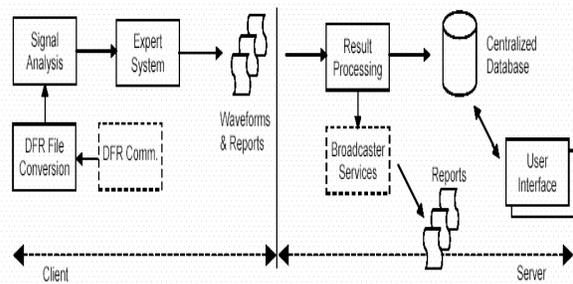
Fig. 2. Digital Fault Recorder Analysis Software Modules
