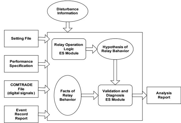
Fig. 1. Digital Protective Relay Analysis Software Modules
