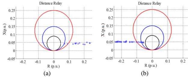
Fig. 4. Distance relays mis-operation, a) overload on line 26-30, b) power swing on line 22-24
