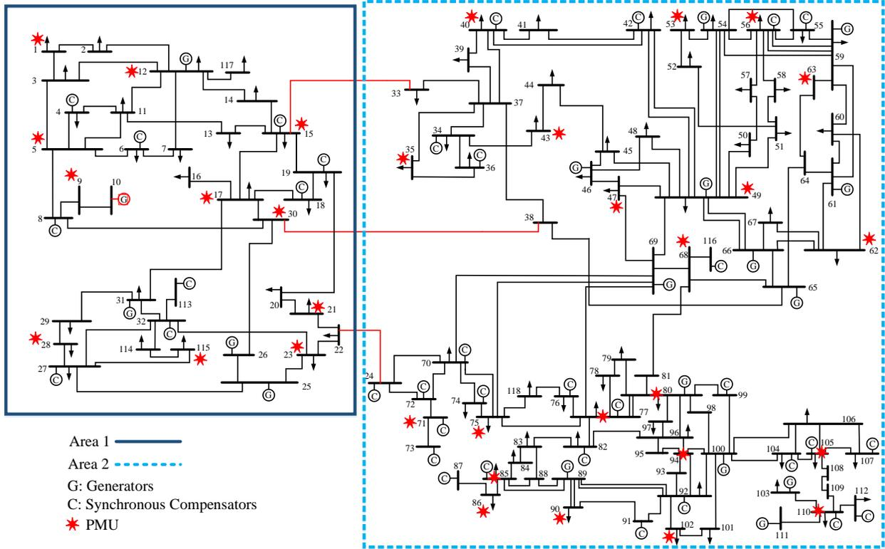
Figure 3. IEEE 118-bus test system
