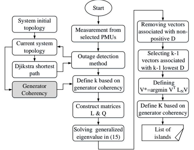
Fig. 2. Flowchart of the proposed cascade event prevention method
