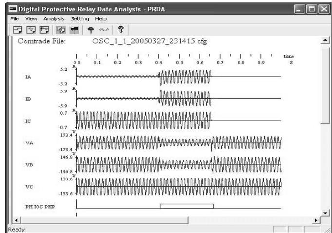
Fig. 6 Oscillography file generated by the relay model
