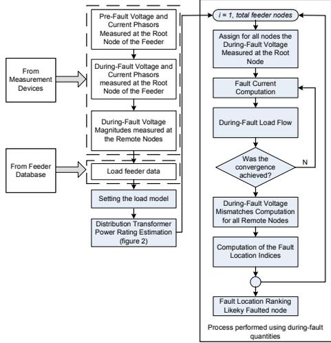
**Figure 1:** Block diagram of the algorithm.
