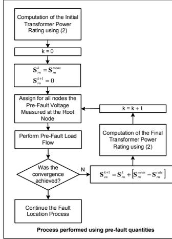
**Figure 2:** Procedure for estimating the transformer power rating.
