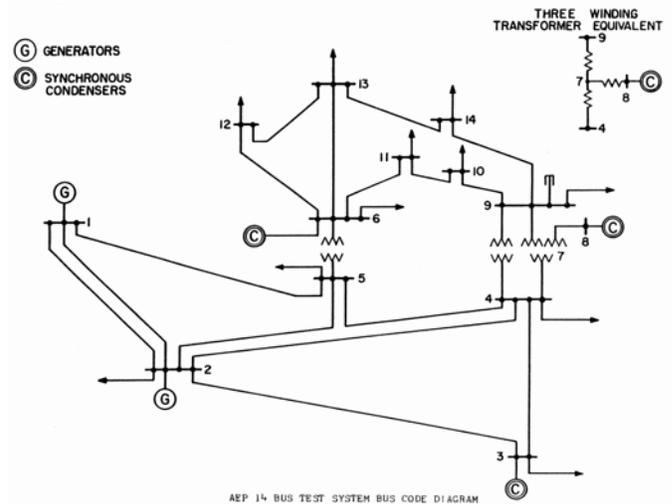
Fig. 2. IEEE-14 bus system diagram.
