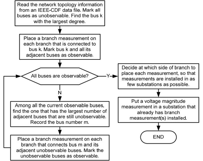
Fig. 1. Flowchart of the branch power flow and voltage magnitude measurement placement.
