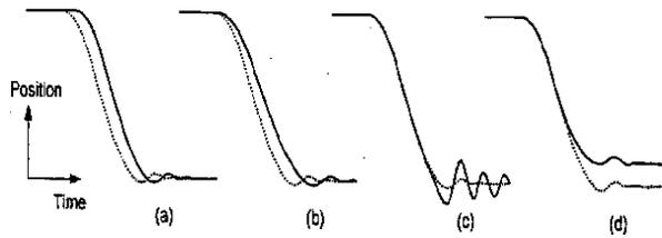
Fig. 2 Comparison of circuit breaker contact travel curves [4]
