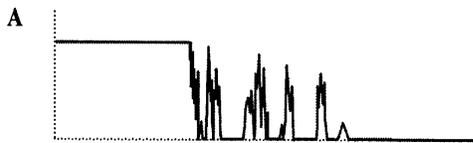
Fig. 5. Noisy transition when opening
