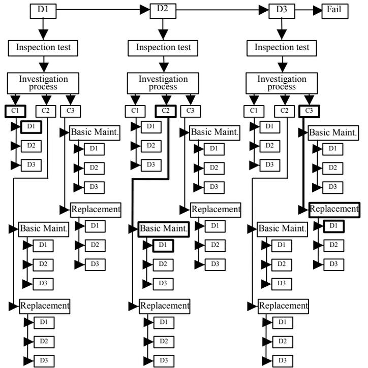
Fig 1. Proposed circuit breaker probabilistic maintenance model.
