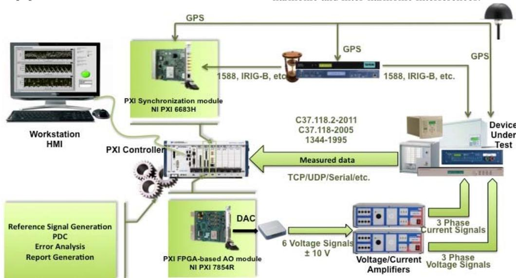
Fig. 1. Calibration and testing platform for PMUs.
