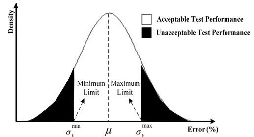
Fig. 3. Probability distribution and the bands assigned to the error indicators for each PMU type-test  $k$ .
