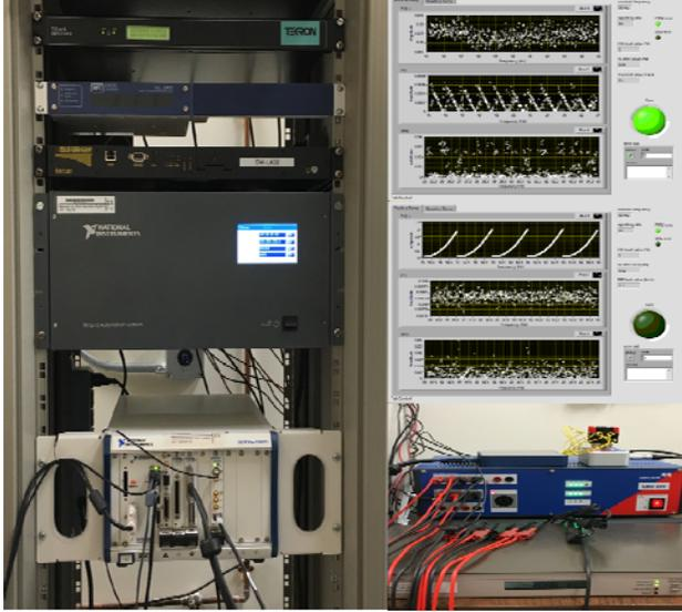
Fig. 2. Actual implementation of the PMU testing platform.
