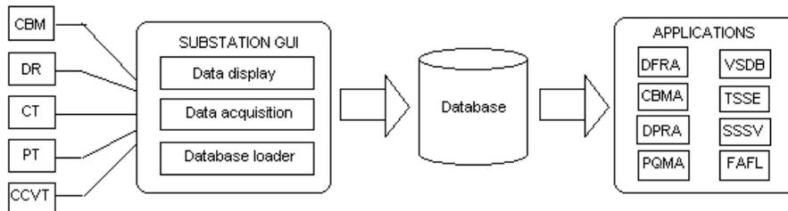
Figure 2 Concept of data integration at substation level
