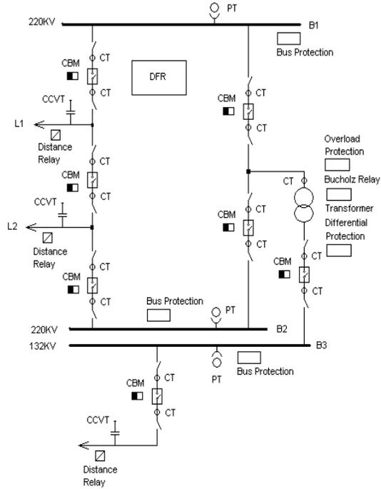
Figure 4 One-line substation diagram
