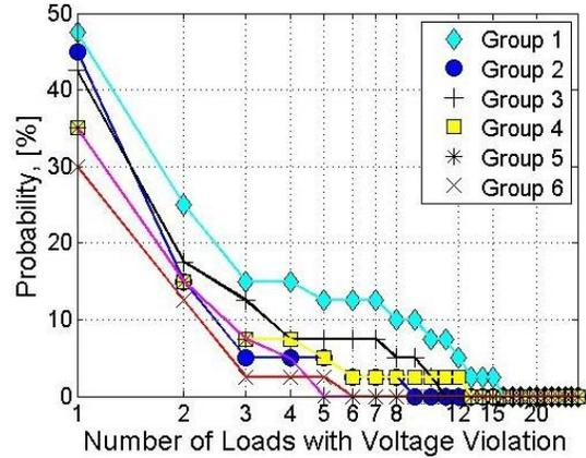
Figure 4. Probability of having voltage violations of more than  $\pm 5$  % versus the number of loads with violation.
