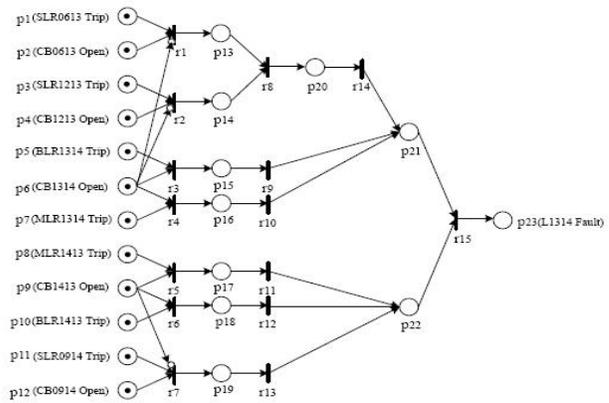
Fig.8. A FRPN model for L1314 fault based on SCADA data
