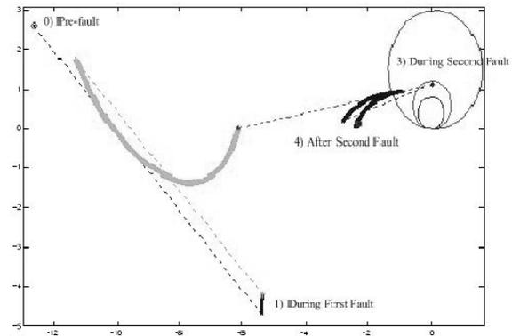
Fig. 6. Apparent impedance seen by distance relay at B26 of L33
