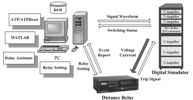
Fig. 3. Test setup for physical relay test
