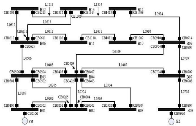
Fig.7. A 14-bus power system model
