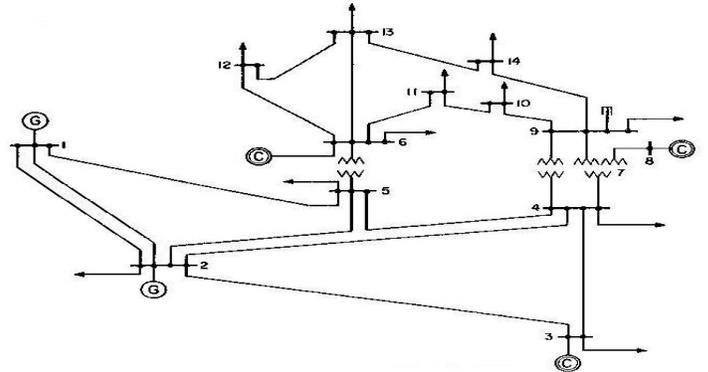
Fig. 2. One line diagram for IEEE 14-bus system
