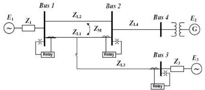
Fig. 1. One line diagram for IEEE PSRC system
