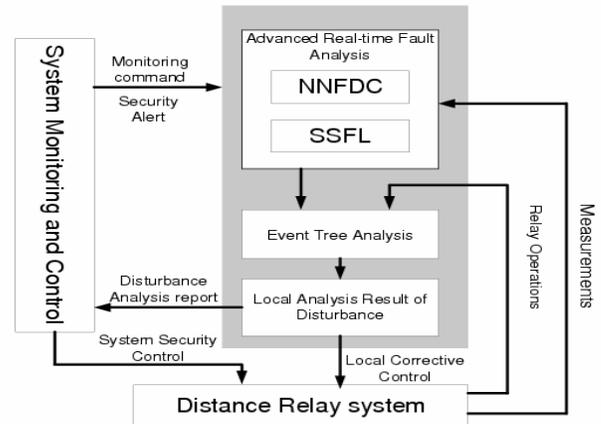
Fig. 4. Block Diagram of Local Monitoring and Control
