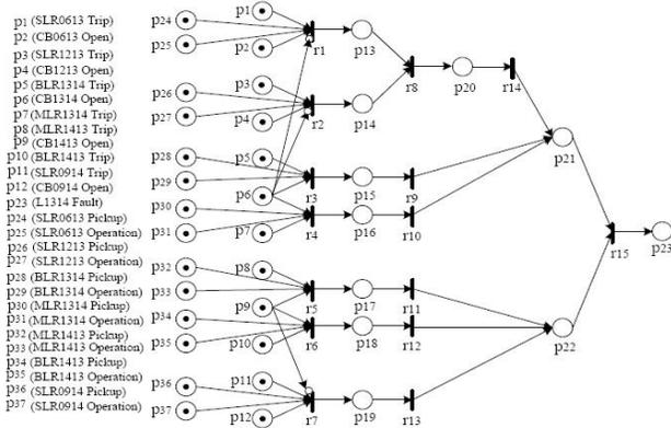
Fig. 9. A FRPN model for L1314 fault based on SCADA and digital protective relay data
