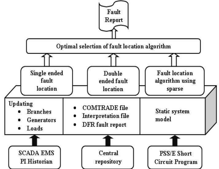
Fig. 9. Architecture of Optimal Fault Location Algorithm
