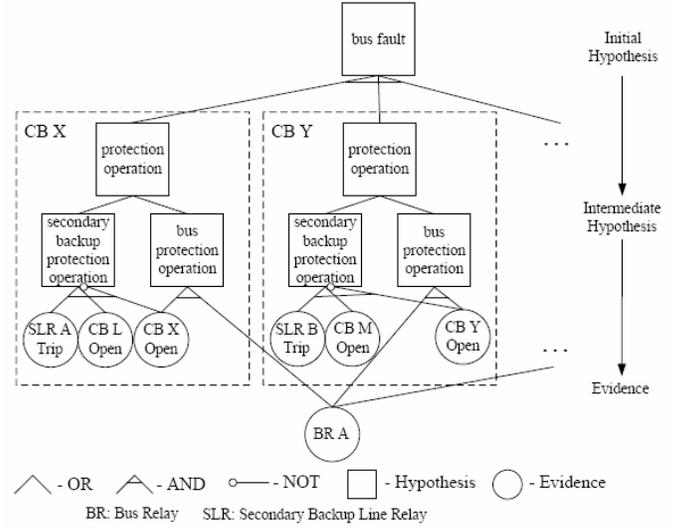
Fig. 5. A FRPN model for L1314 fault based on SCADA and digital protective relay data
