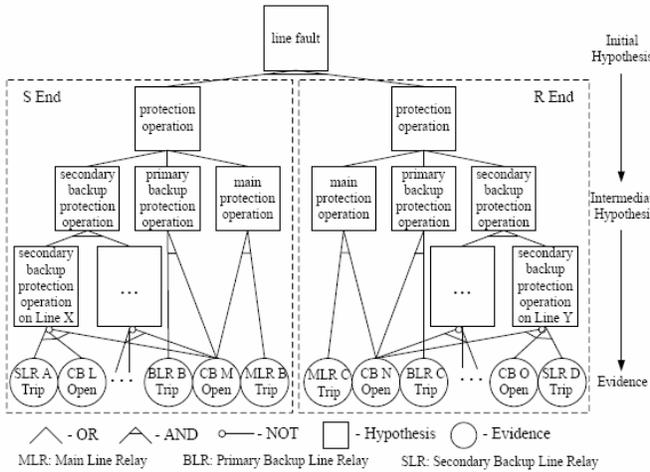
Fig. 4. Backward Reasoning concept for structuring transmission line diagnosis models
