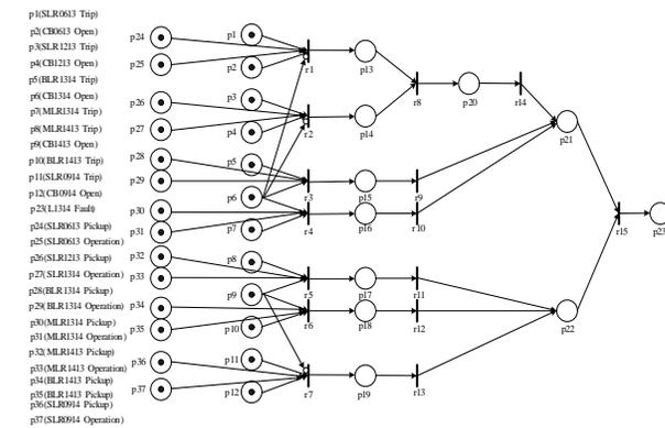
Fig. 7. A FRPN model for L1314 fault based on SCADA and digital
