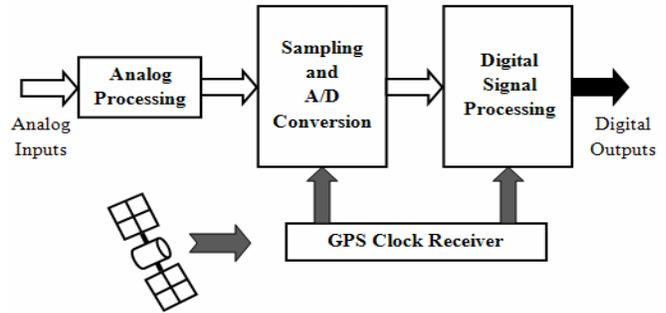
Fig. 1. Data Processing in IED
