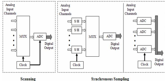
Fig. 2. Scanning and synchronous sampling of analog inputs
