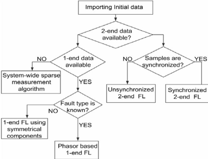
Fig. 8. Flowchart of Optimal Fault Location Algorithm
