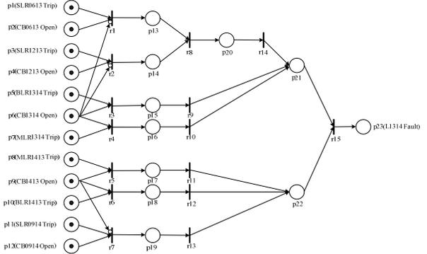
Fig. 6. A FRPN model for L1314 fault based on SCADA data
