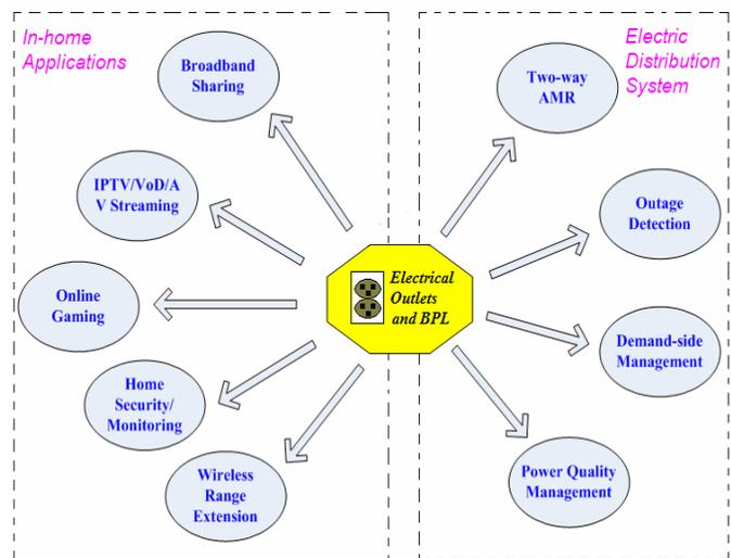
Fig. 1. Various services that can be provided using BPL technology
