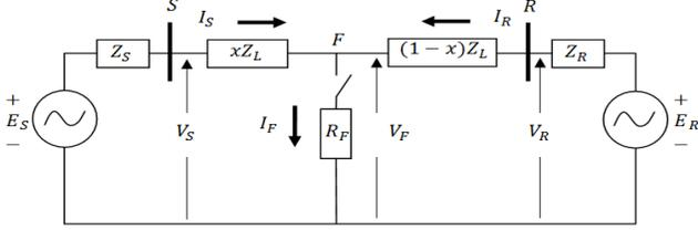
Figure 1. Faulted circuit model
