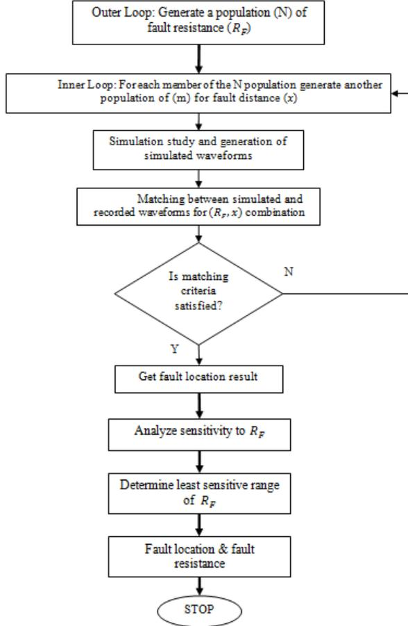
Figure 3. Flowchart of corrected sparse measurement algorithm
