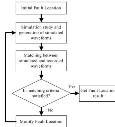
Figure 2. Flowchart of sparse measurement algorithm
