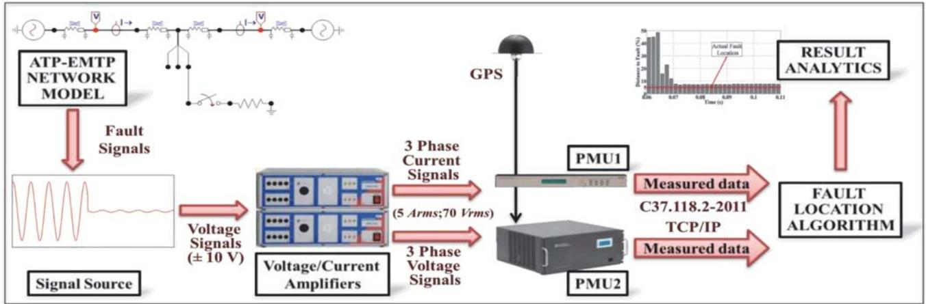
Fig. 2. Synchrophasor-based testbed set up for evaluation of the impact of PMU errors on the end-use applications.
