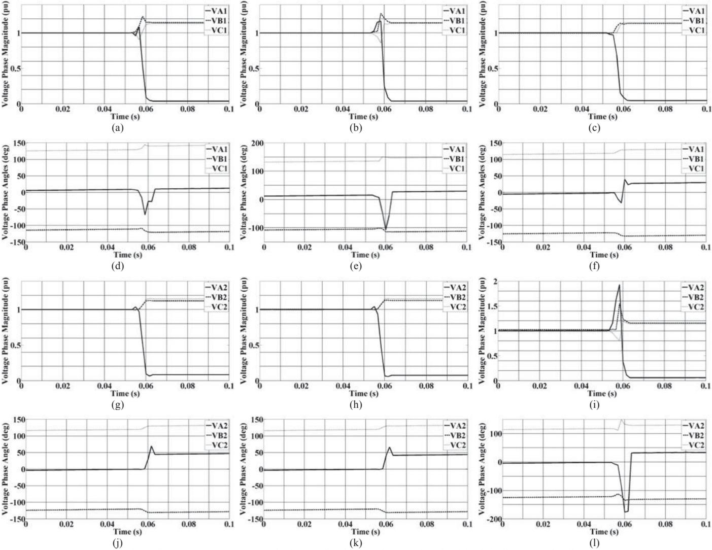
Fig. 4. PMU measurements: magnitudes and the phase angles at both ends of the faulted transmission line.
