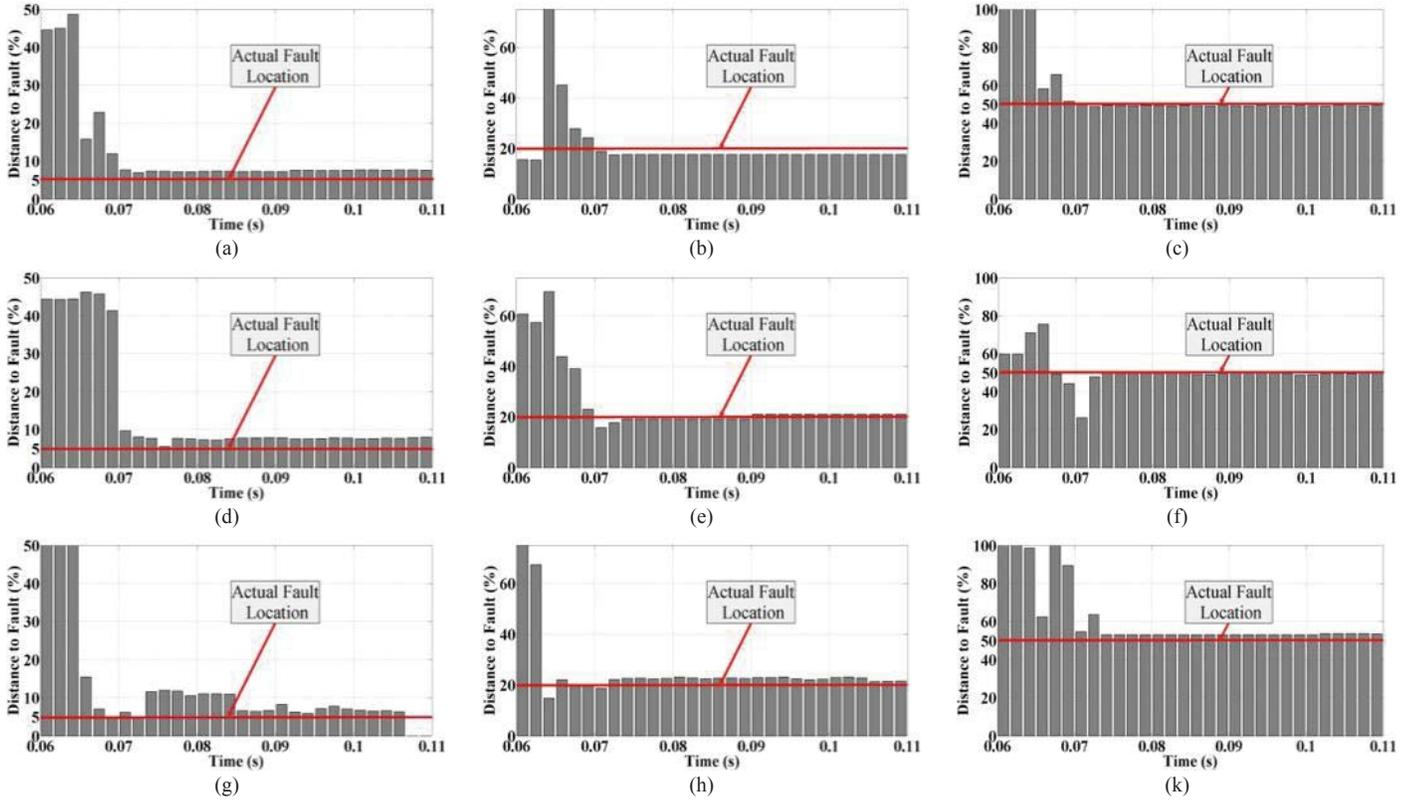
Fig. 5. Synchrophasor-based fault location algorithm performance: calculated fault locations for different fault use case scenarios.
