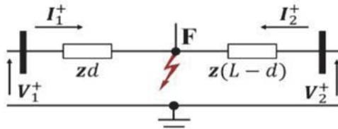
Fig. 1(b). Equivalent positive sequence network of the faulted TL.
