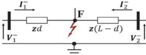
Fig. 1(a). Equivalent negative sequence network of the faulted TL.
