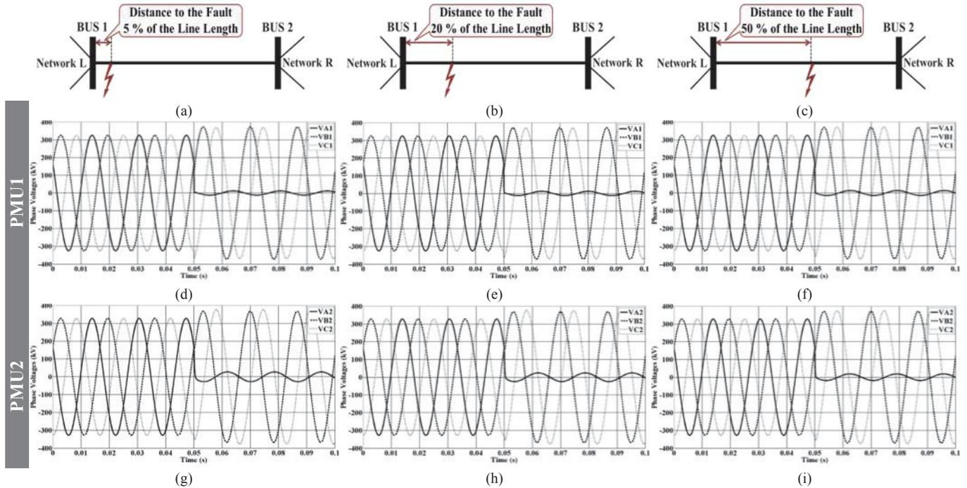
Fig. 3. Simulated phase voltages in the transmission line fault use case scenarios.
