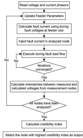
Figure 2. Flow chart for voltage sag based fault location method.
