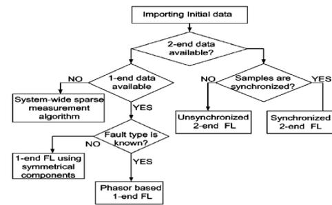
Figure 1. Flowchart of Optimized Fault Location Algorithm [9].
