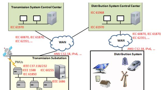
Figure 4. Standard related to transmission and distribution fault location applications.
