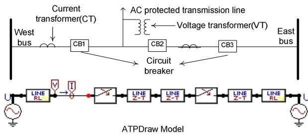
Figure 4. Power system model for simulation
