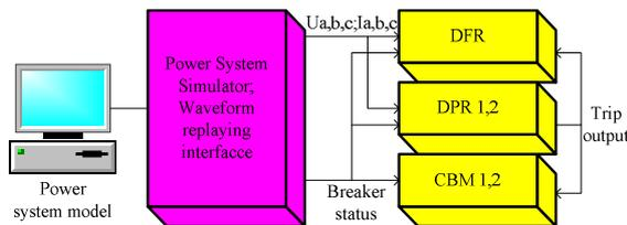
Figure 5. Simulation system structure
