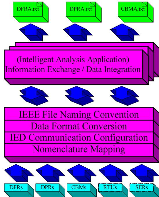
Figure 1. Automated integration and analysis of IED data
