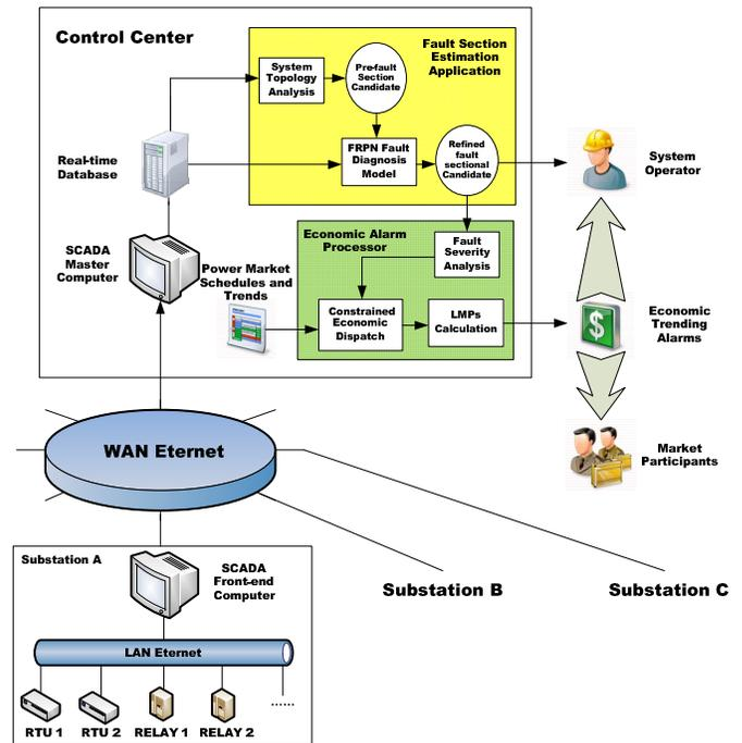
Fig. 8. Intelligent Economic Alarm Processor Architecture
