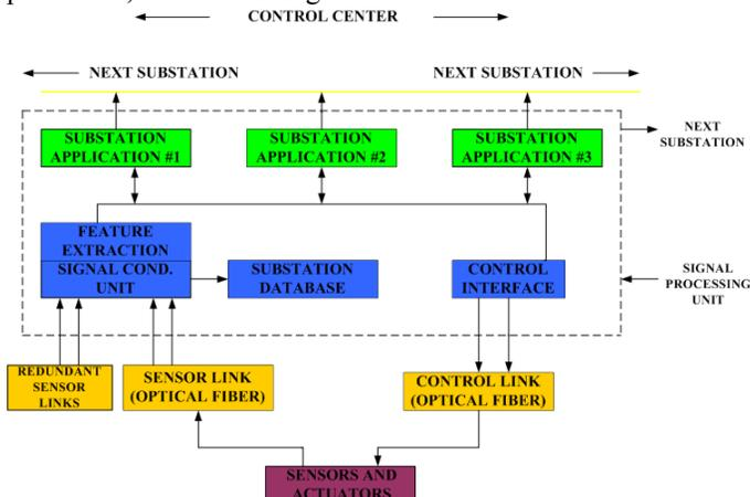
Fig. 5. Architecture of new monitoring and control network
