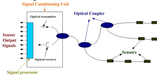
Fig.2. Multiplexing arrangement for FFPI sensors
