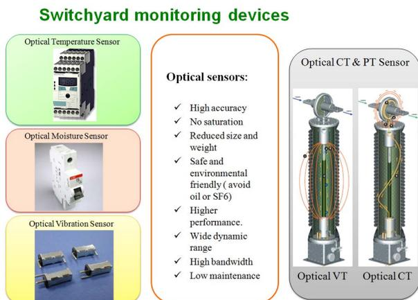
Fig. 4. Switchyard monitoring devices
