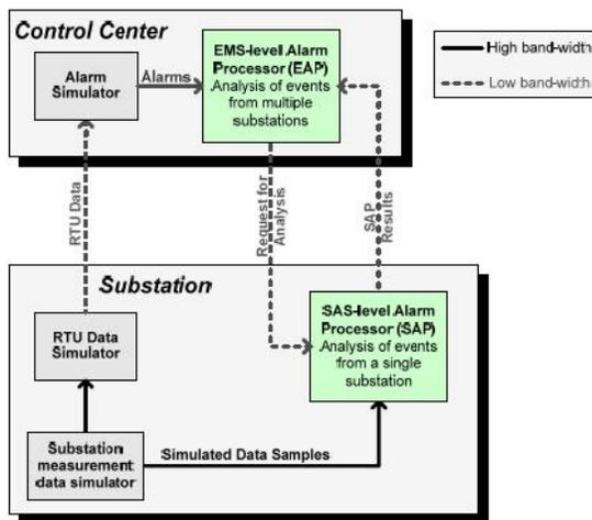
Fig.3. Overall Software Structure
