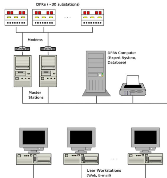
Fig. 1 DFR system for automated fault analysis
