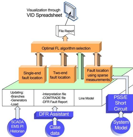
Fig. 8 Architecture of proposed solution
