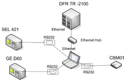
Fig. 5 IED data synchronization
