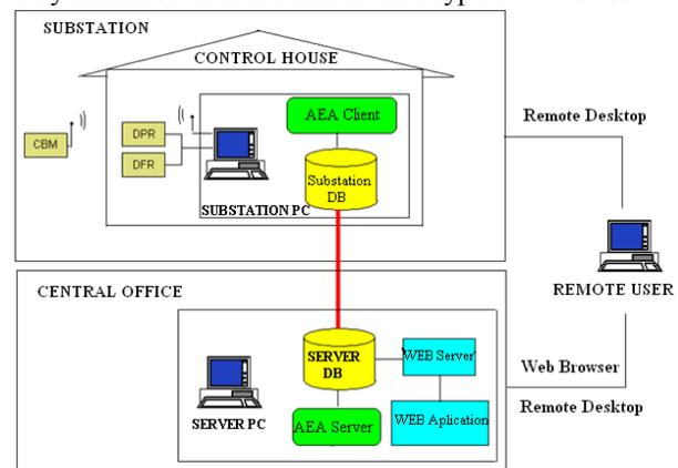
**Fig.9. Software architecture for substation automation**
