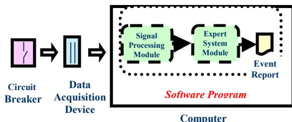
**Fig.10. CBM hardware and software**
