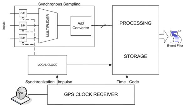
Fig.1. Synchronized sampling implementation
