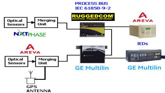
Fig.2. Typical optical transformer configurations
