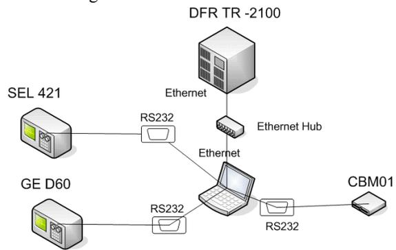
**Fig.8. Connections of IEDs in a substations**
