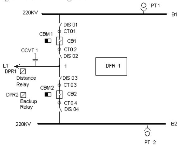
**Fig.7. One line diagram of a portion of a substation**
