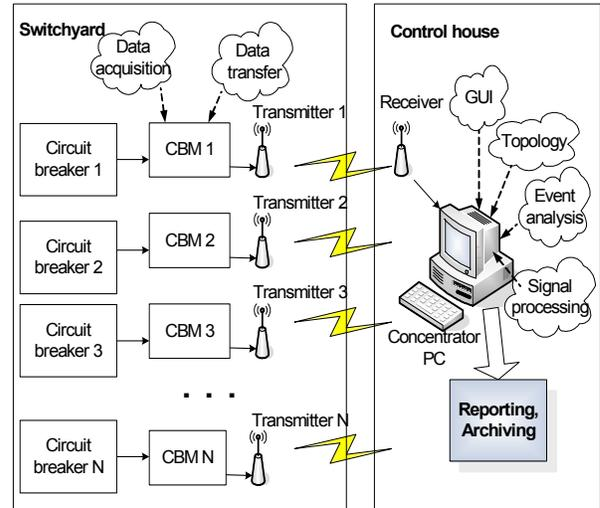
**Fig.11. Monitoring of a sequence of CB operations**
