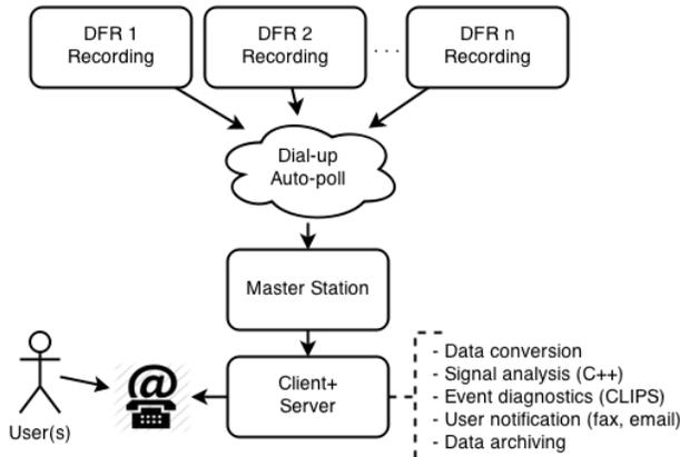
Fig. 4. Centralized system solution using dial-up (~30 DFRs)
