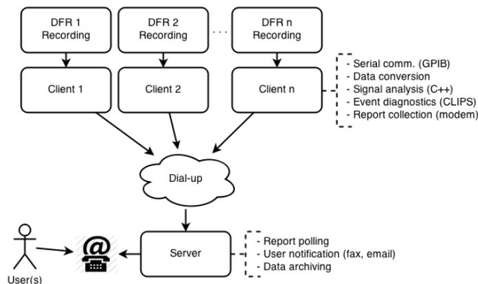
Fig. 3. Decentralized system solution using dial-up (~10 DFRs)
