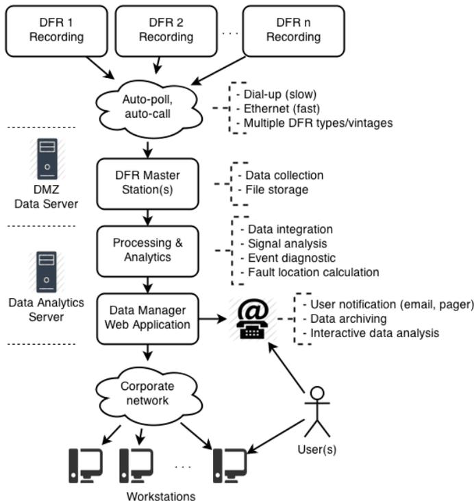
Fig. 5. Full-blown centralized system solution (~ 100 IEDs)
