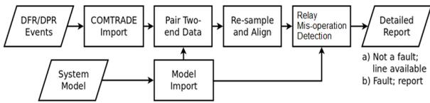
Figure 8. Automated analysis of time-synchronized event data
