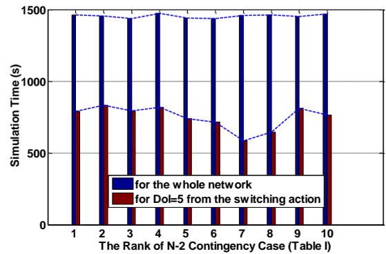
Figure 9. Simulation time with and without implementing DoI
