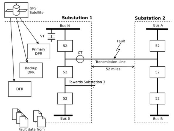
Figure 7. Transmission line setup with measurements from both ends
