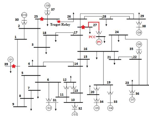
Figure 10. New-England 39 bus system with DG penetration
