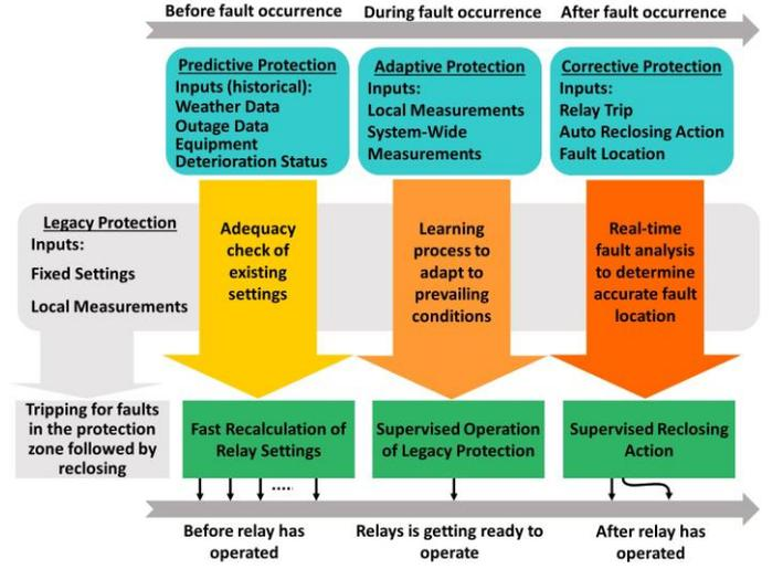
Figure 2. Legacy distance protection supervised by HCP
