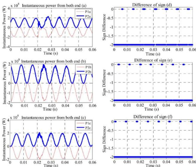
Figure 12. Detection of relay misoperation
