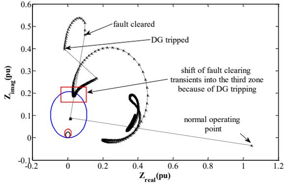
Figure 5. DG tripping impact on apparent impedance trajectory
