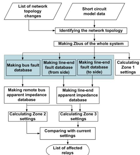
Figure 4. General flowchart of the settings calculation module
