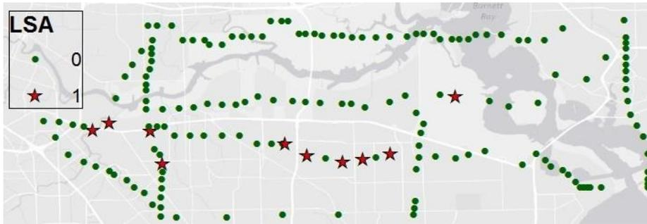
Fig. 5. Optimal locations of line surge arresters based on risk analysis.
