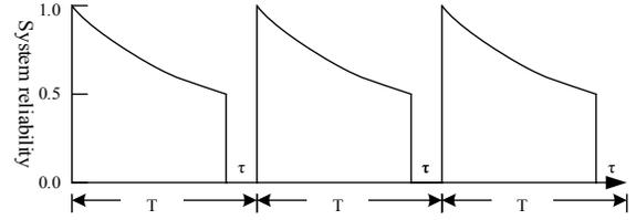
Fig. 3. System reliability of the protection system with periodic inspection.
