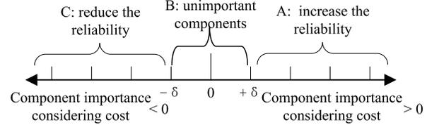
Fig. 8. Application principles of component importance considering cost.
