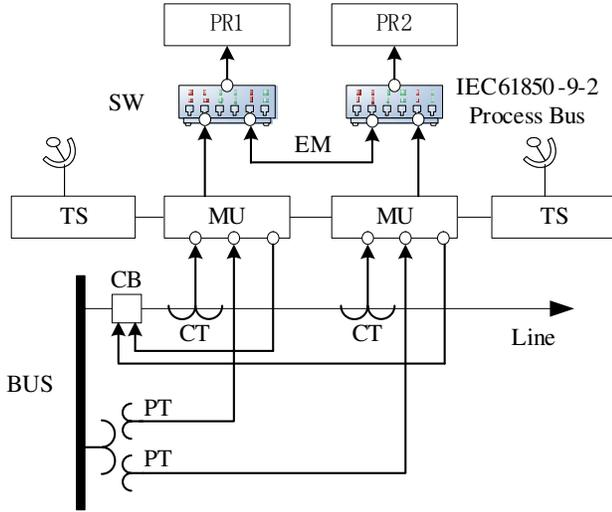
Fig. 1. A typical architecture of the all-digital protection system.
